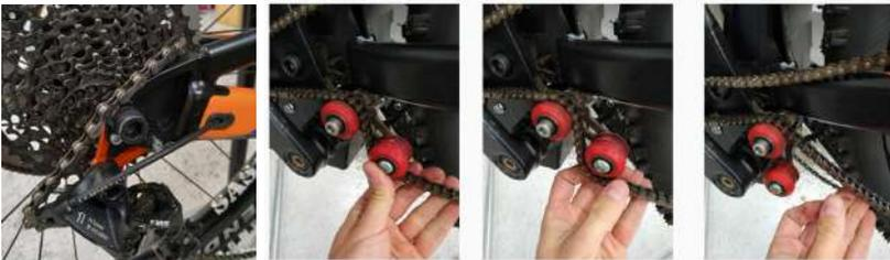
3. Install the engine chain over the swingarm.
