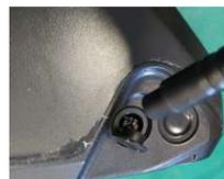
To install the battery on the frame, slide it back into the U-channel of the frame and be sure to do so when the battery is completely at the bottom. A click indicates that the battery is locked in place.
