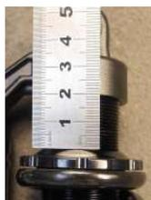
The spring preload is done with a hook wrench or by hand.
