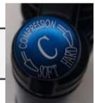
When adjusting, it is best to turn the button until the soft stop and then adjust the desired position. The factory setting is 3 notches from the "soft" stop (fully unscrewed thumbwheel).
